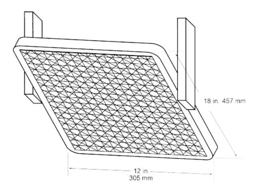
Figure 3b - Air Propane Radiant Panel
