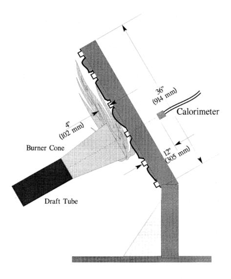
Figure 6 - . Position of Backface Calorimeters Relative to Test Specimen Frame
