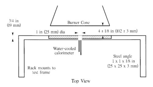
Figure 4 - Calorimeter Position Relative to Burner Cone
