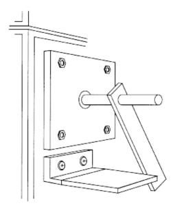
Figure 8 - Propane Burner Stop
