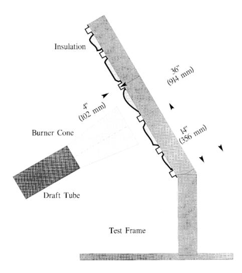
Figure 2 - Burnthrough Test Apparatus
