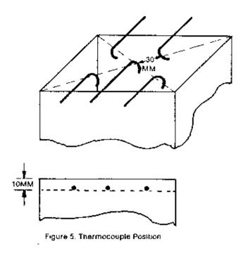
Part V. Test Method To Determine the Smoke Emission Characteristics of Cabin Materials
