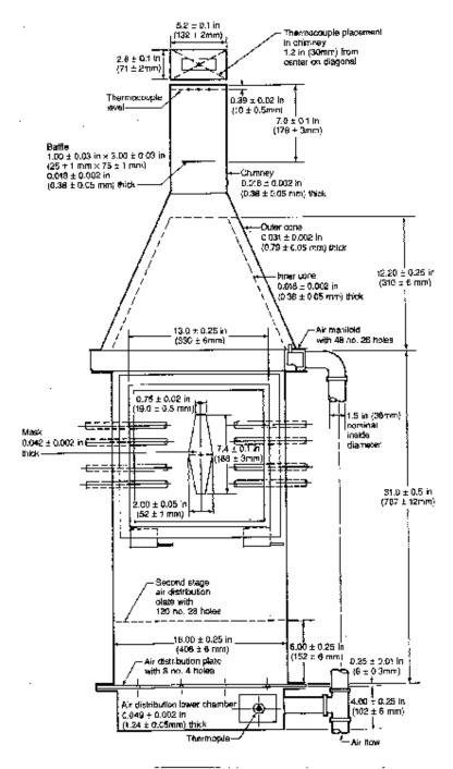
Figure 1A Rate of Heat Release Apparatus
