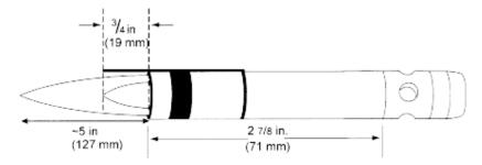
Figure 6 - Propane Pilot Burner
