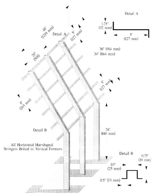
All Material 0.125" (3 mm) Thickness Except Center Vertical Former, 0.250" (6 mm) Thick
