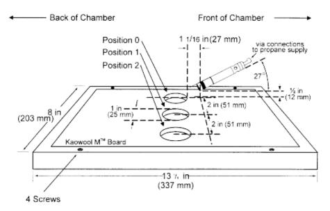
Figure 7 - Calorimeter Holding Frame
