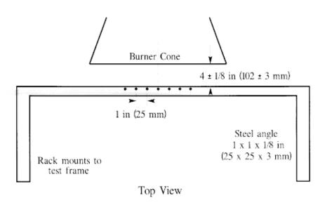
Figure 5 - Thermocouple Rake Position Relative to Burner Cone
