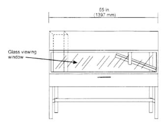
Figure 1 - Radiant Panel Test Chamber
