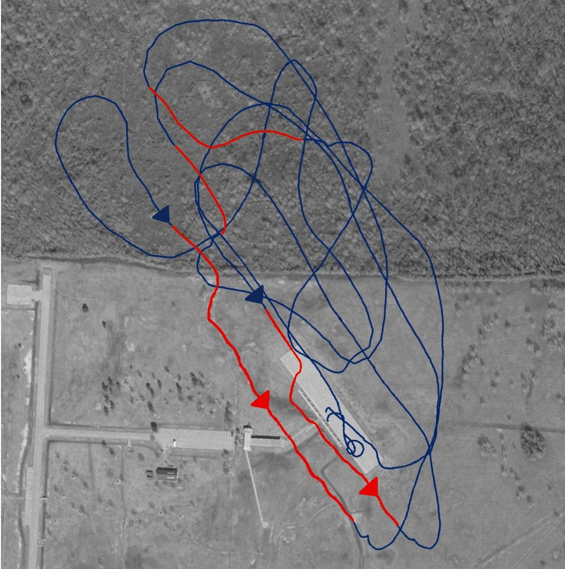
Figure 4.2: Plot of plane's trajectory during the second flight test on 04/02/2011. The red lines indicate parts during which the autopilot was active. Arrows on the line segment indicate the plane's direction of travel.
