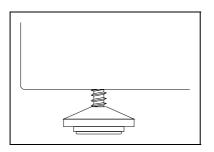
• Two spacers attached to the appliance must be fitted onto the upper edge of the condenser, thus preventing the appliance from being installed too close to the wall. Spacers are manufactured for all-purpose function depending on the distance of the condenser from the wall. Therefore turn spacers correspondingly and fix them to the appliance.
