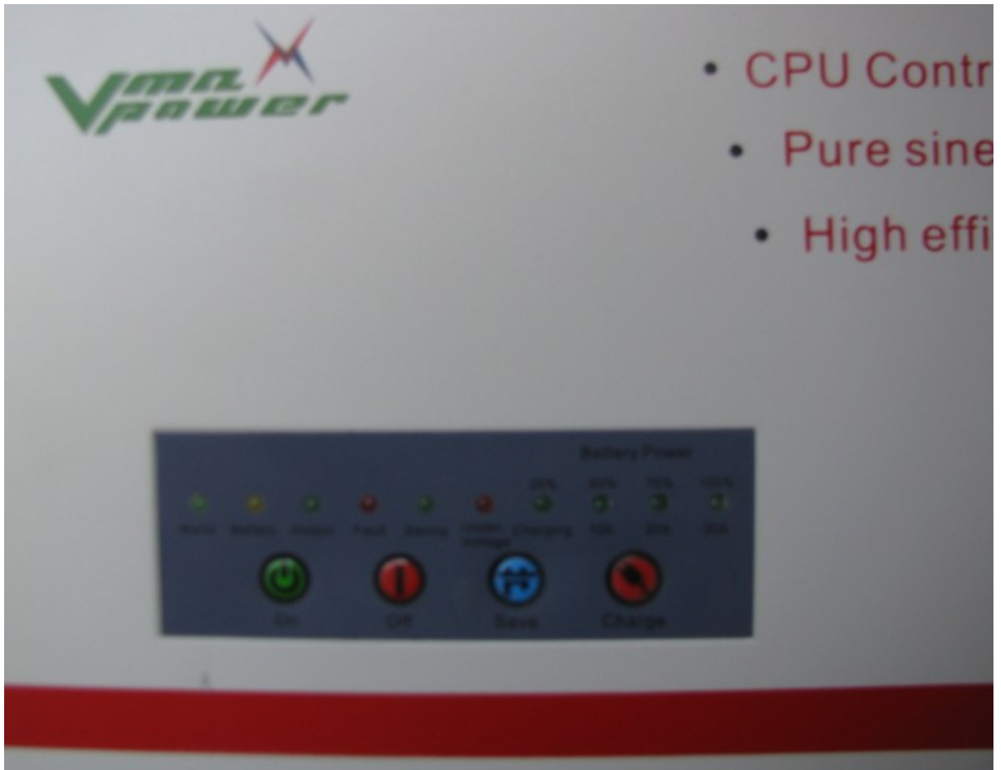
LCD control panel of inverter
