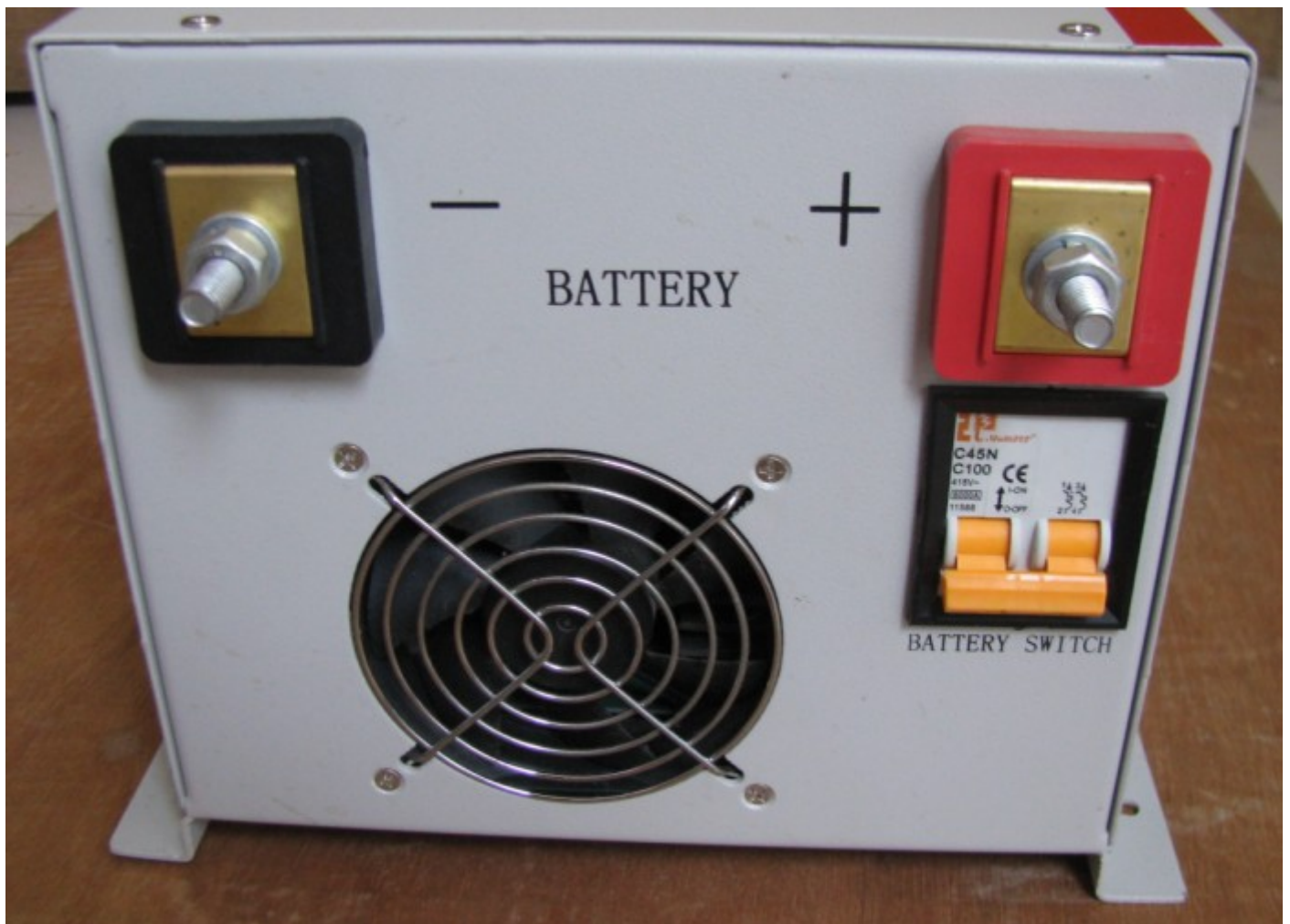
Battery terminals of inverter
