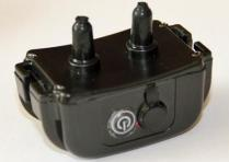
4) Test the shock of the collars by using the wire shock tester. Wrap the wires around the 2 metal posts of the collar then press the shock button. The bulb will light up if the collar is giving a shock.
