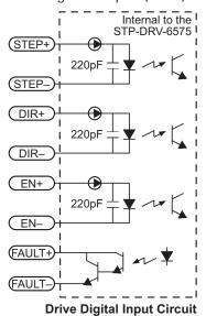
The digital inputs are optically isolated to reduce electrical noise problems. There is no electrical connection between the control and power circuits within the drive, and input signal communication between the two circuits is achieved by infrared light. Externally, the drive's motor power and control circuits should be supplied from separate sources, such as from a step motor power supply with separate power and logic outputs.
