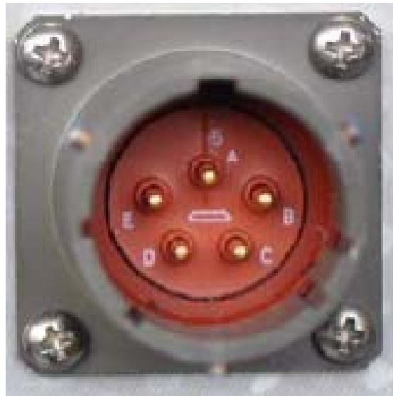
Figure 1: Labeled Pins in the Power Cable Port
