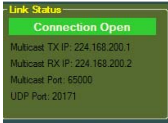
Figure 17: Quasonix Remote Terminal Window, Link Status Box
