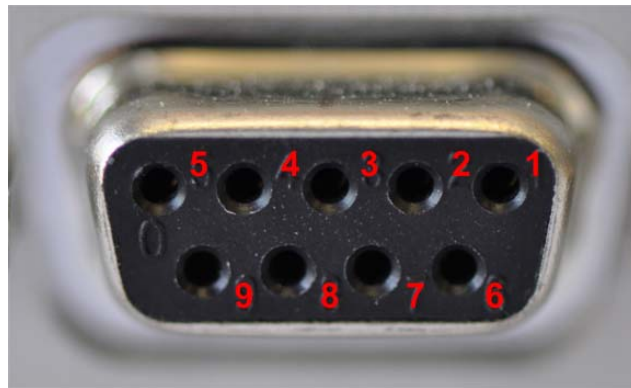
Figure 6: Front Panel DB-9 Serial Port Pins Labeled
