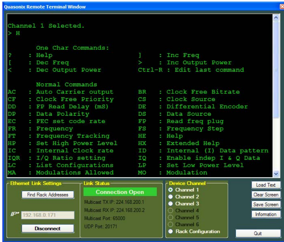
Figure 20: Quasonix Remote Terminal Window, Channel 1, Transmitter Command List
