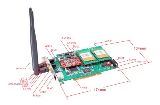
GX01: GSM module, one GX01 supports one GSM channel.
