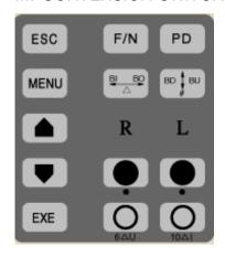
These switches are for parameter-conversing, inputting a program. (Refer "setting up on P 14.).
