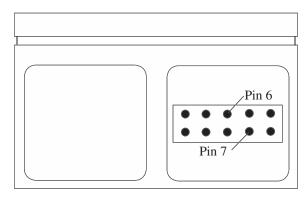
To apply the 1 Vdc signal to the calibrator connect the precision voltage generator so that the positive line is connected to Pin 7 and the ground is connected to Pin 6.
