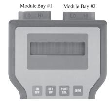
**Step 1** Remove any installed measurement modules. If the CQS calibration module is to be used, install it in module bay #1 at this time.
