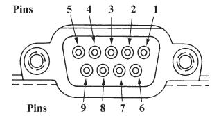
Pin 8 Relay 2 common Pin 9 Relay 2 (normally opened or normally closed)
