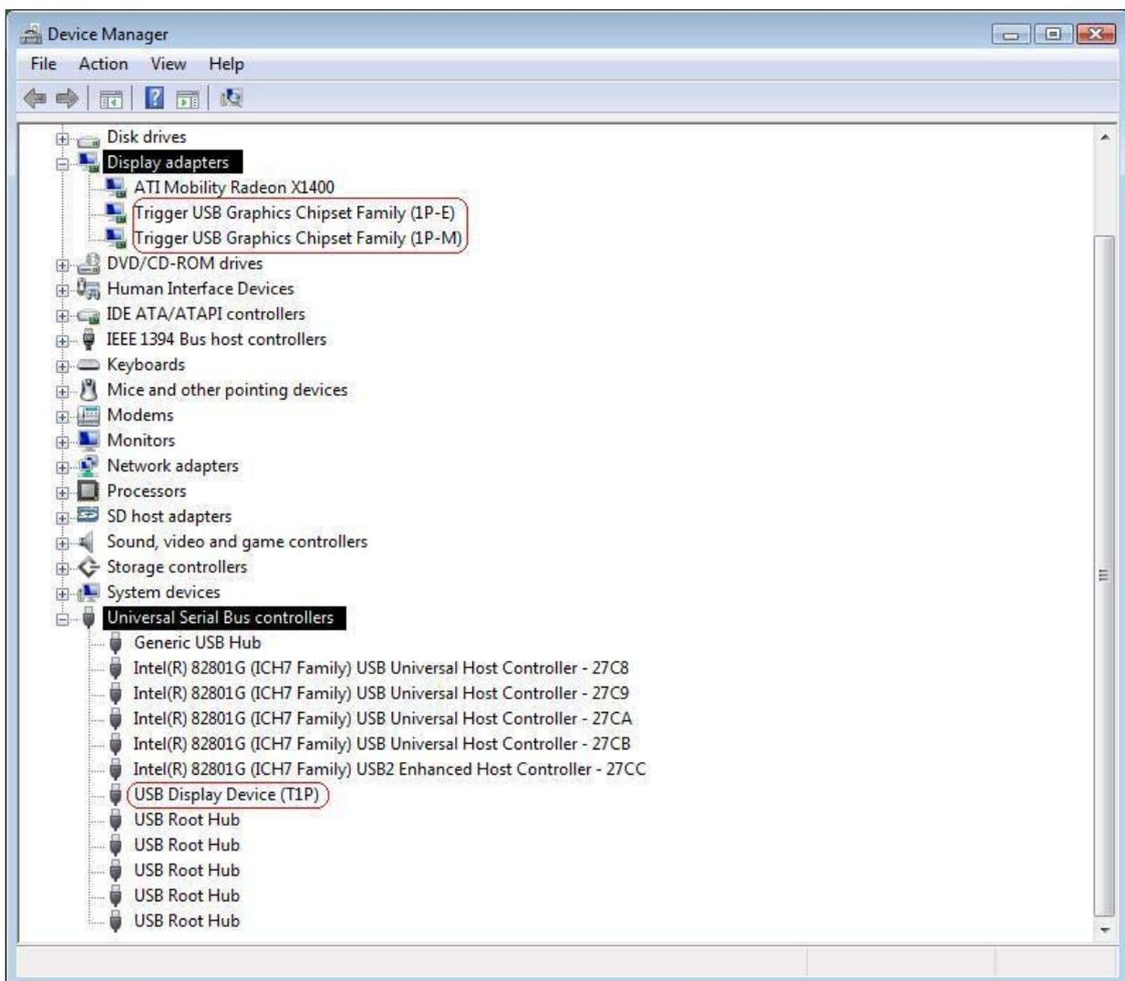
Begin verification by make sure highlighted devices were added to the system. (Multiple USB Display adapters)
