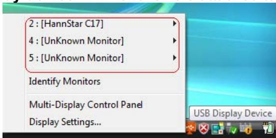
If there is no display device attached to the USB to WSXGA+ Adapter, an “**Unknown Monitor**” ID will be shown. In some cases, the attached display device does not support EDID, the ID will also be defined as “**Unknown Monitor**”.
