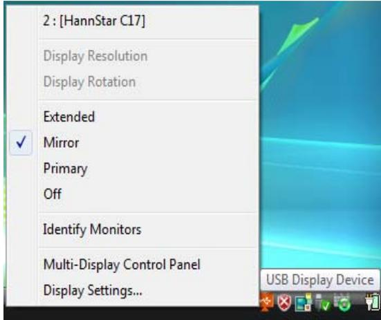
The screen resolution setting on the USB Display enabled device will follow the on-board screen's resolution. For example, if the on-board screen's resolution is 1024x768x32bit, and the USB Display enabled device will set as the same resolution.
