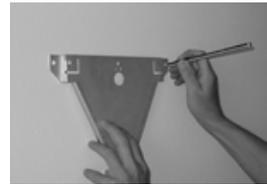
At this point detach the panel from the body of the instrument. After to have connected supply and sensors, insert the body into the support and fix using two lateral screws.
