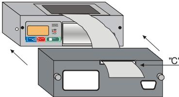
Insert paper into slot "C" and replace the panel in its original position. Cut off excess paper. (for further details on "Paper feed" see Chapter 6)
