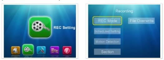
At the "**Rec mode**" screen, press "▲▼" to select "**Cam 1-2-3-4**", and press "◄ ►" to select "**Motion/Manual/Schedule**", then press "**Enter**" to confirm and press "**Menu**" to exit.
