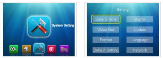
At the "**Date & Time**" screen, press " $\checkmark$   $\blacktriangleright$ " to select "**DATE**" and "**TIME**", then press " $\blacktriangle$ " to select digital "0 - 9 ","DATE" and "TIME", then press "**Enter**" to confirm and press "**Menu**" to exit.
