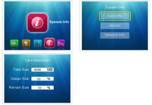
Remarks: this operation is to check the SD card total capacity and the percent of the used and the rest capacity,
