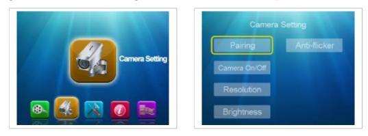
5.1.1.3 At the "**Pairing**" screen, press the "**Enter**" to enter next step, and press "▲ ▼" to select "**Cam 1-2-3-4**", and press "**Enter**" to confirm, then press "**Pairing**" button at the back of camera within **30 seconds** to finish pairing.
