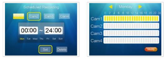
Remarks: date/hours in yellow means the settings are finished, and press "Menu" to exit.
