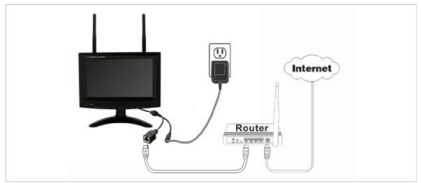
Lock the LCD DVR on the bracket and install the antenna to the LCD DVR, connect the RJ45 network cable between LCD DVR and Router, then plug and turn on the power adapters of LCD DVR and Router.
