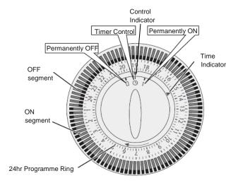
Timer control segments 1 segment = 15mins OFF – Segments on inside of ring ON – Segments on outside of ring
