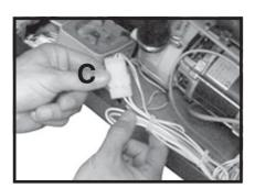
Connect the plug (C) of the wire harness with the dosage pump (max. 100 VA).
