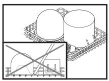
Close door and push the ON button ①, tank will be filled.
