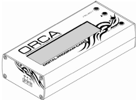
Connect the battery wires to a charged pack of battery. Turn on the ESC and the setting card will activate automatically. Note that the screen will show "Loading..." during initialization – indicating that the ESC is copying the current setup in the ESC to the setting card. Once loading is completed, the screen will show "ORCA VRITRA-VTC - Program". You can now start to program your ESC.
