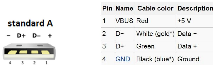
Figure 15. USB 1.x/2.0 standard pinout 19
