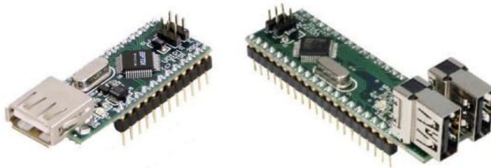
Figure 2. VDIP1 (left) and VDIP2 (right) with VNC1L 3
