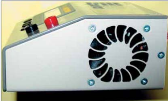
Left side: laser cut cooling holes
