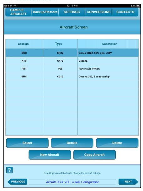
The Aircraft Screen is used to select an aircraft for the flight. No aircraft are pre-defined in the Flight Planner aircraft database so initially this screen will show no aircraft. Aircraft can also be defined, copied, modified or deleted from the aircraft screen.
