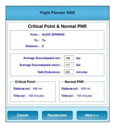
Critical Point and Point of No Return can be displayed for each flight stage. Enter the groundspeeds for the outbound and return sectors, and the safe endurance, and press the *Recalculate* button.
