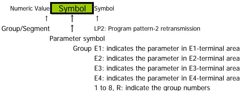
Display may be controlled according to the setting value of the setup parameter and operation status.
