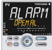
3. Press the SET/ENTER key to display the [A1] Parameter Setting Display.
