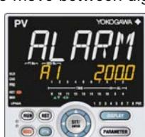
6. Press the SET/ENTER key to register the setpoint (the setpoint stops blinking).
