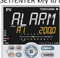
7. Press the PARAMETER key once to return to the Menu Display. Press the DISPLAY key once to return to the Operation Display.
