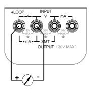
Press the key (OUTPUT/IN/SW) when the OUTPUT appears in the display. It denotes that the calibrator is in an output state.
