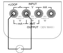
2) When the key (**OUTPUT / IN/ SW**) is pressed, the display indicates the symbol 'INPUT' followed by the word 'CLOSE' or 'OPEN' according to the measured switching contact status.
