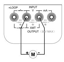
2) When the key (**OUTPUT** / **IN/SW**) is pressed, the display indicates the symbol 'INPUT'. It denotes that the calibrator is in an input state.
