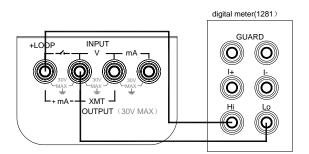
Press the keys (POWER), (OUTPUT / INPUT/SW) and (mA%/V) simultaneously to enter the calibrator in a state of 20mA output calibration, and then the symbols (OUTPUT), (CAL 0', (ON) and (mA' appear in the display.
