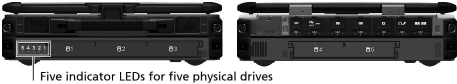
You can easily swap a drive by loosening the screws to open the protection door and then pulling the drive out of its slot.
