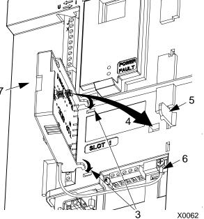
**NOTE!** Correct installation of the ground lead is essential for fulfilling the EMC requirements and for proper operation of the module.
