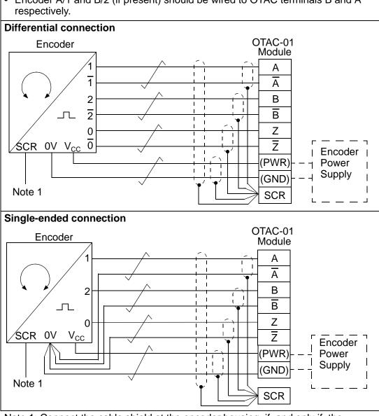
Note 1: Connect the cable shield at the encoder housing, if, and only if, the encoder is isolated from the motor, and from ground.
