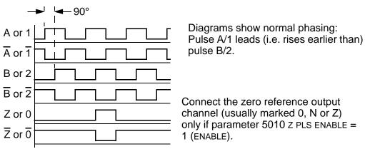
The encoder output channel that leads when the drive runs *Forward* should be connected to OTAC terminal A. The output channel that trails should be connected to OTAC terminal B.
