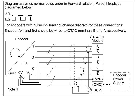
Note 1: Connect the cable shield at the encoder housing, if, and only if, the encoder is isolated from the motor, and from ground.
