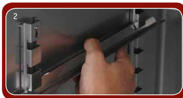
2 Install Shelf Slide (#5121028) by aligning with Shelf Standards (#5170646) at a slight upward angle and set into a level position.
