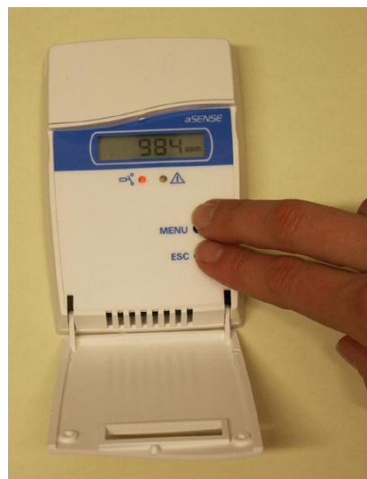
Figure 11 The ENTER command is done by pushing buttons MENU and ESC at the same time for about 14 seconds
