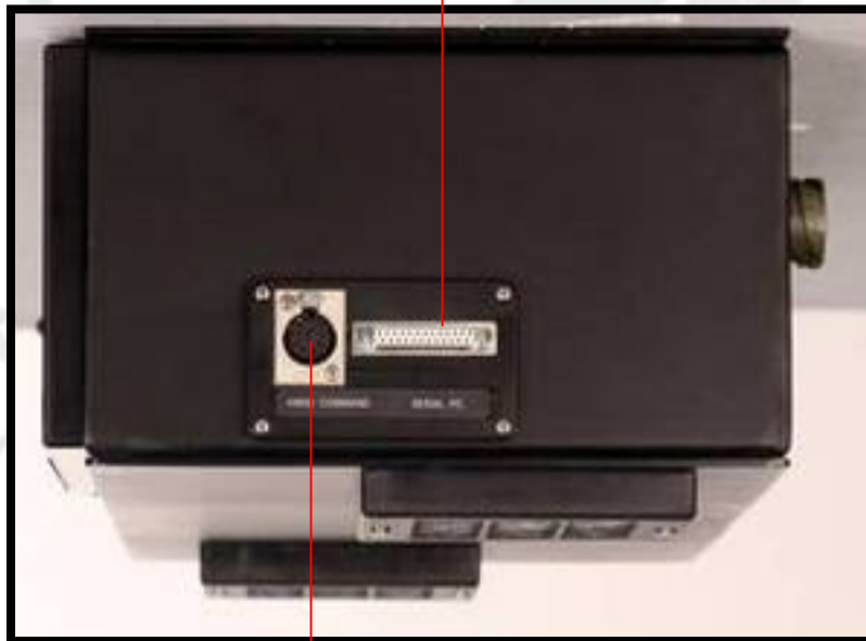
Hand command's connector - NEUTRIK 7pins panel female NC7FP1
