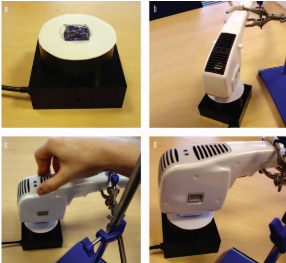
Figure 1. (A) Mask the absorber head with a white PTFE sheet with aperture exposed for energy collection; (B) fix the applicator in place on the absorber head energy collection aperture using a laboratory retort clamp and stand; (C) take fluence measurements with the applicator transmission block flat and central on the absorber head energy collection aperture; (D) apply firm downward pressure to eliminate air bubbles and tighten clamp fixing.
