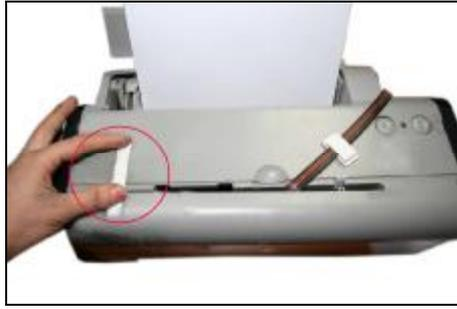
Close the front cover with a sticky tap and avoid the tube being clamped tightly.
