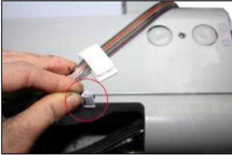
Insert a scrip in the proper position of printer top cover as the picture shown above.
