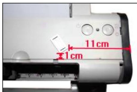
Fix the supporting arm as the picture shows. Measure 11 cm from the right edge of printer, 1 cm from the below edge, which forms an angle of 60°.
