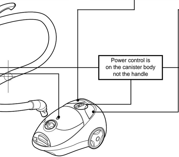
Power control is on the canister body not the handle
