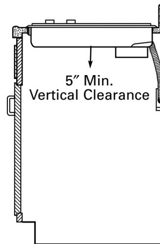
Make sure the wall coverings, countertop and cabinets around the cooktop can withstand heat up to 200°F (93°C) generated by the cooktop.
