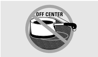
Always center the pan on the surface element you are using.
