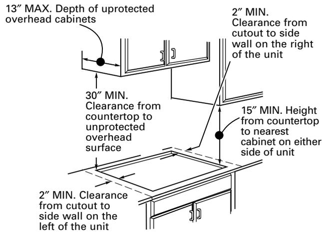
If a 30-inch clearance between the cooking surface and overhead combustible materials or metal cabinets cannot be maintained, a minimum clearance of 24 inches is required and the underside of the cabinets above the cooktop must be protected with not less than ¼-in. insulating millboard covered with sheet metal not less than 0.0122 inches thick.
