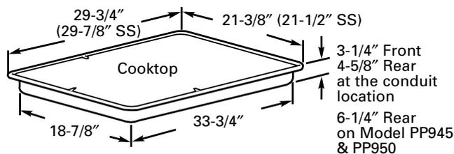
There must be 5 inches minimum vertical clearance between the cooktop bottom and any combustible surfaces.
