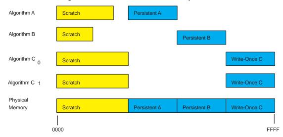
Figure 2-1. Scratch vs Persistent Memory Allocation
