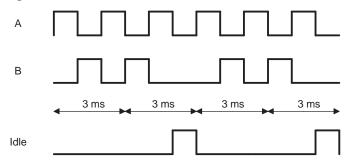
In this case, both task A and B meet their deadlines and we have more than 18% (1 ms every 6 ms) of the CPU idle.
