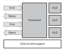
Figure 1-2. DSP Software Architecture
