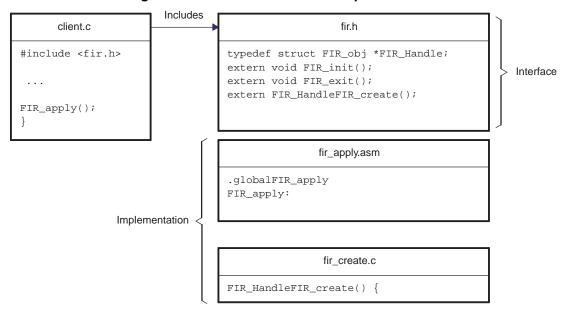
Figure 3-1. Module Interface and Implementation
