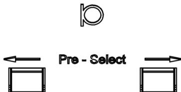
Press the left or right PRE SELECT button to scroll through a list of all available output channels. The list is shown in the top line of the display. The language channels are coded according to the international MARC language codes. You may then select and assign a channel out of all available channels.
