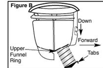
Remove insect debris from screen surrounding funnel. Wash screen with water and shake off excess water before re-installing.
