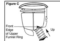
Push funnel upwards and with the rear section of the bottom funnel ring at a slight angle compress funnel until front tabs of bottom funnel ring are up inside of the housing. See figure D.
