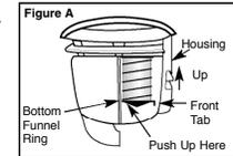
Pull funnel down and forward releasing rear section of upper funnel ring and remove funnel from unit. See figure B.
