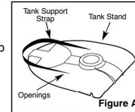
On the underside of the tank stand, loosen the two hex nuts located on the screws which extend from the sides of the base plate. Place the slots at the ends of the tank support strap over the screws and secure by tightening the two nuts. See Figure B.
