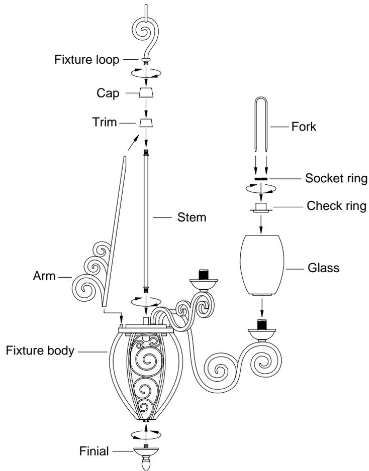
1. Before beginning the assembly, carefully unpack and identify all parts referring to the illustration.
