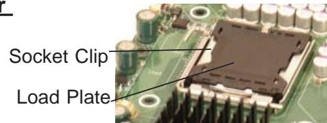
1. Press the socket clip to release the load plate, which covers the CPU socket, from its locking position.
