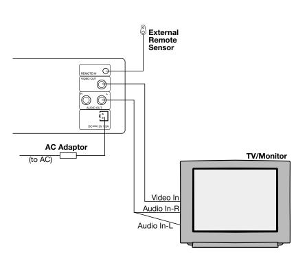
Set the unit. You have to set the unit according to the TV/monitor to be connected.
