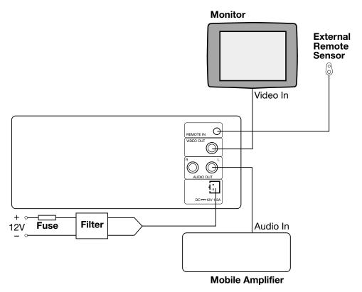
In the connection diagram, the system's power leads should be connected at the same point to minimize noise.
