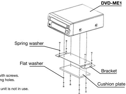
Fix the \_\_\_\_\_ bracket to the unit with screws.
