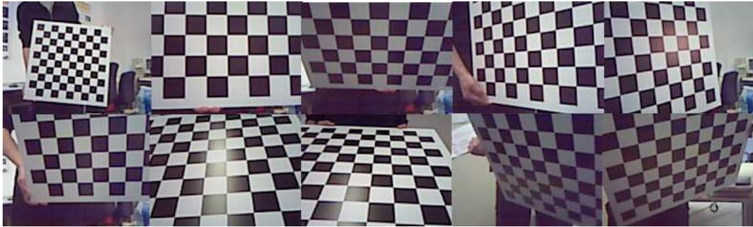
Figure 5.1: The images used in the camera calibration
