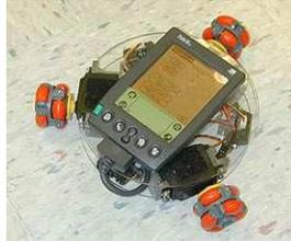
Figure 2.7: Palm Pilot Robot with omniwheels
