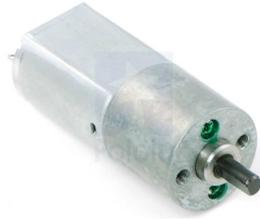
Figure 3.4: Pololu 25:1 Metal Gearmotor 20Dx44L mm. Key specs at 6 V: 500 RPM and 250 mA free-run, 20 oz-in (1.5 kg-cm) and 3.3 A stall.
