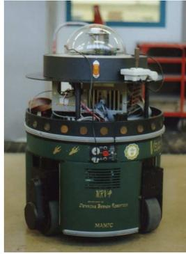
*Figure 2.6: MRV4 robot with synchro drive mechanism*
