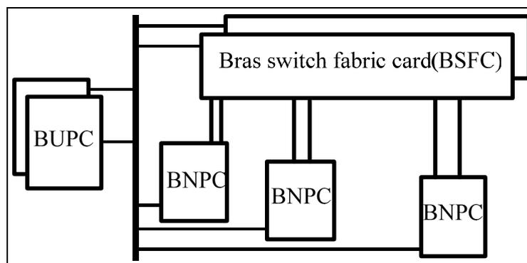
Serial high-speed signal line is used between BSFC3 and each BNPC. 100BASE-TX communication control signal line is used for connection with BUPC.
