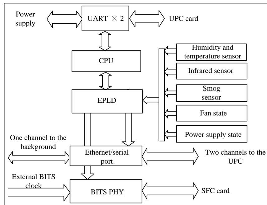
**Smog Sensor** Smog sensor on BIC generates current signals once it detects smog, and then card converts current signals into level signals, which is sent to EPLD.
