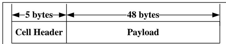
**Virtual Circuit** ATM is a connection oriented switch technology based on virtual circuit. Each virtual circuit is identified VPI (Virtual Path Identifier) and VCI (Virtual Channel Identifier). Each VCI or VPI only has local meaning on the link between ATM nodes.
