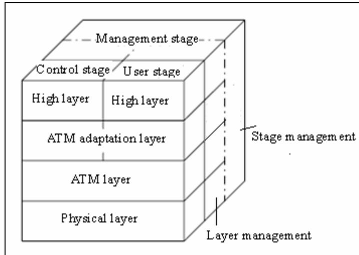
AAL (ATM Adaptation Layer) is the interface connecting high layer and ATM layer. It forwards information between high layer and ATM layer. There are four types of AALs: AAL1, AAL2, AAL3/4 and AAL5. Each type of AAL supports some different types of services in ATM network.
