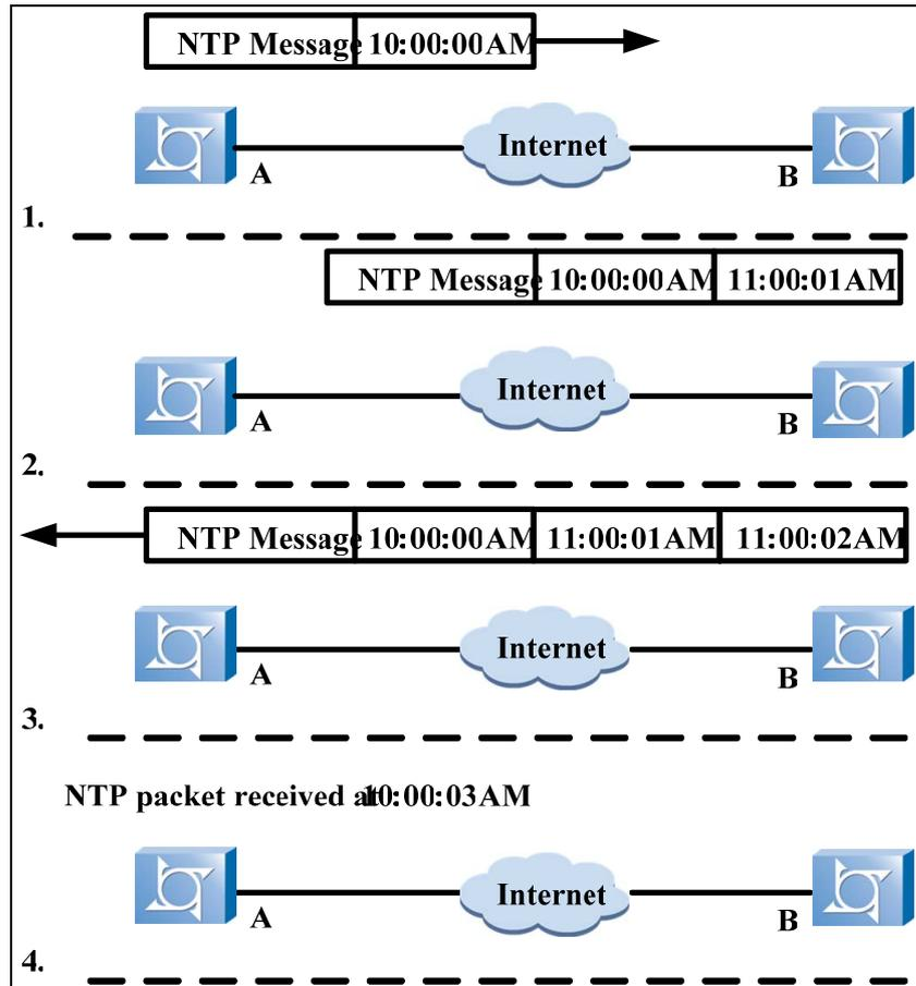
In Figure 50, devices A and B are connected through serial interface. Both devices have their own system clock independently. It is to synchronize the two system clicks now. Suppose:
