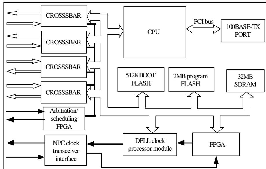
ZXUAS 10800E Carrier Class BRAS, switching of IP packets is conducted by CROSSBAR chip on BSFC and high-speed serial backplane chip on BNPC. CROSSBAR chip has following functions and features:
