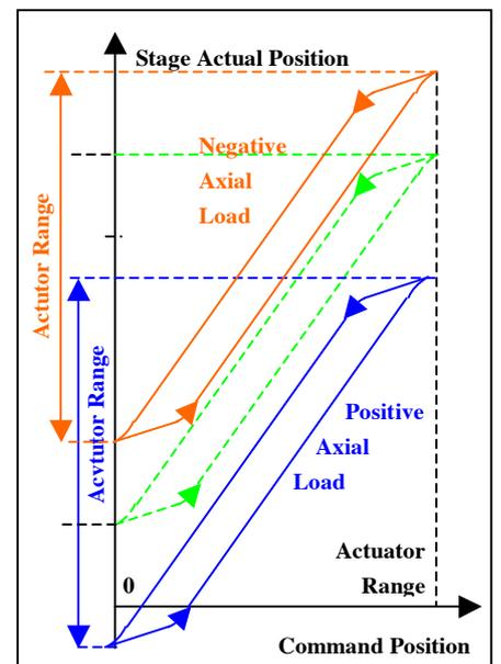
Figure 2 : Open loop, with axial load
