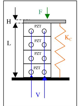
**Note:** The piezoelectric principle is reversible, by applying a force to this crystal; it creates a voltage difference between the ends.
