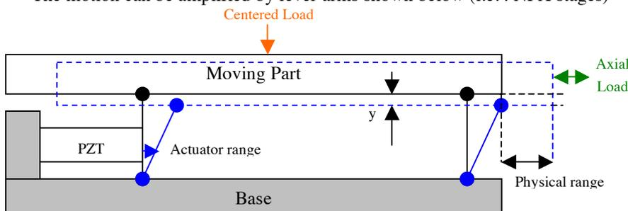
**Note:** The design of the stage mechanism is important to minimize the motion in the orthogonal dimension (y) which can be neglected.
