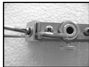
Screw sealing wire down under a clamp plate.
