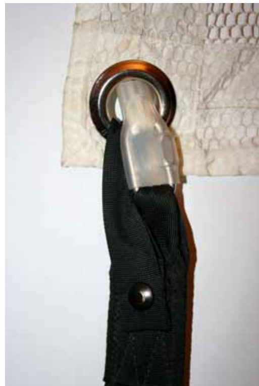
Figure 2a & Figure 2b: Attaching the slider down retainer strap
