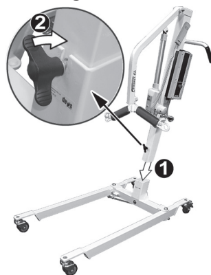
Inserting the mast
