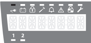
C4UC0201 Control Panel It has 2 Zones or Inputs that are shown in the lower part of the display.
