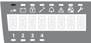
C4UC0401 Control Panel It has 4 Zones or Inputs that are shown in the lower part of the display.
