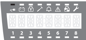
C4UC0801 Control Panel It has 8 Zones or Inputs that are shown in the lower part of the display and can be grouped into Areas (maximum 4).
