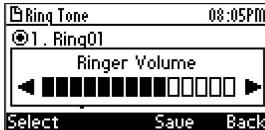
Once you have completed adjusting the volume level, the Ringer Volume indication is hidden after a few seconds.
