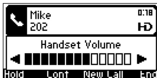
3. Adjust the volume using the ▲ and ▼ VOLUME keys. After you have completed adjusting the volume, the Handset Volume level bar no longer appears on the screen.
