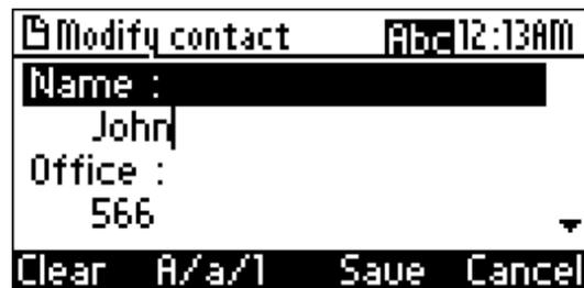
4. Modify the contact's details as required, and then press the **Save** softkey to save your settings.
