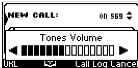
3. Adjust the volume using the ▲ and ▼ VOLUME keys. After you have completed adjusting the volume, the Tones Volume level bar no longer appears on the screen.
