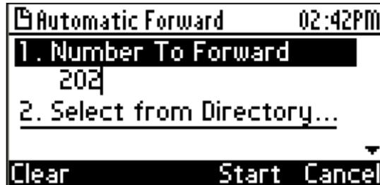
5. Press the **Start** softkey to activate call forwarding; the **Call Forward**
