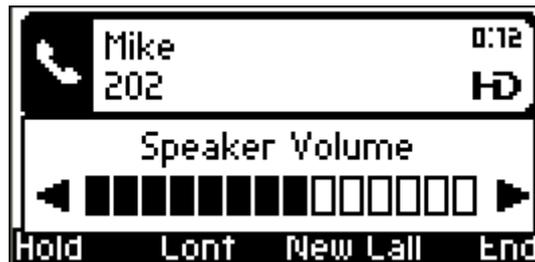
3. Adjust the volume using the ▲ and ▼ VOLUME keys. After you have completed adjusting the volume, the Speaker Volume level bar no longer appears on the screen.
