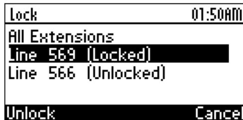
2. Choose an extension (or **All Extensions** to unlock all extensions) that you want to unlock, using the ▲ and ▼ Navigation keys, and then press the **Unlock** softkey; you are prompted to enter the unlock password, as shown below:
