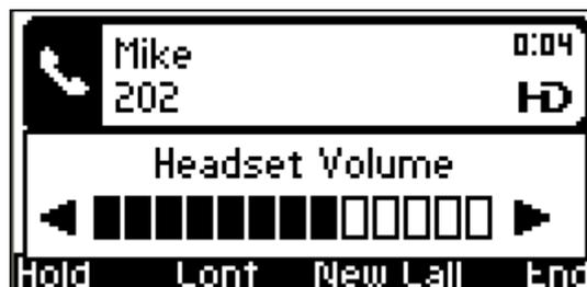
3. Adjust the volume using the ▲ and ▼ VOLUME keys. After you have completed adjusting the volume, the Headset Volume level bar no longer appears on the screen.
