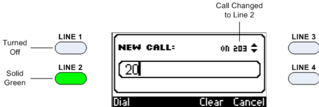
2. Enter the phone number or select the contact from the phone directory, and then press the **Dial** softkey; the phone calls the dialed number and the line on which the call is made is indicated in the screen, as shown below:
