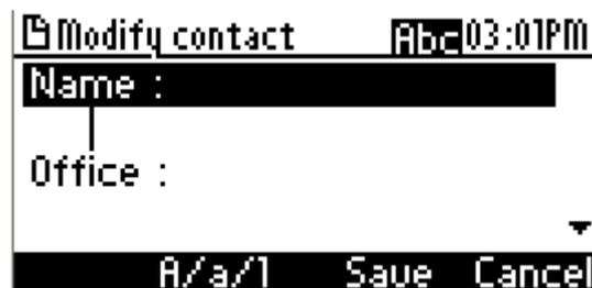
3. Select the 'Name' field (using the **▲** and **▼** Navigation keys), and then enter the name of the new contact.
