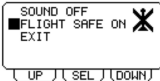
Press **SEL** to turn **FLIGHT SAFE** mode “**ON**”
