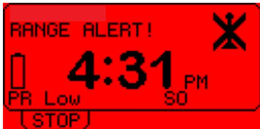
**RANGE ALERT** – Display flashing RED and audible buzzer alert sounding
