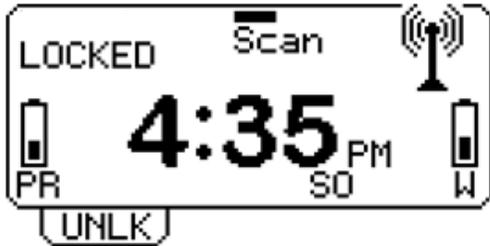
Follow the following steps on the Portable RF Receiver to request a location (WRU) Press **UNLK** to unlock the keypad
