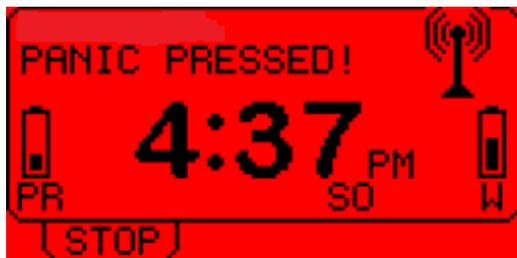
The audible alert buzzer can be stopped by pressing **STOP** on the main screen
