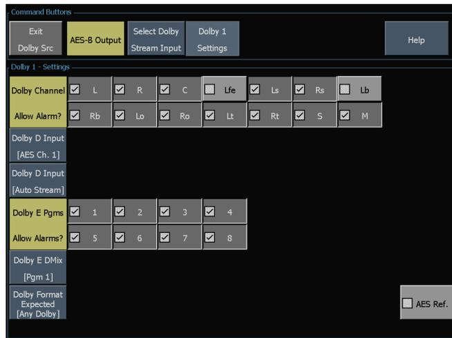
9. **Option DD only:** Select and configure the **Output Map** to assign a specific bar pair to the Analog and Digital Outputs. The outputs are limited to a single pair.
