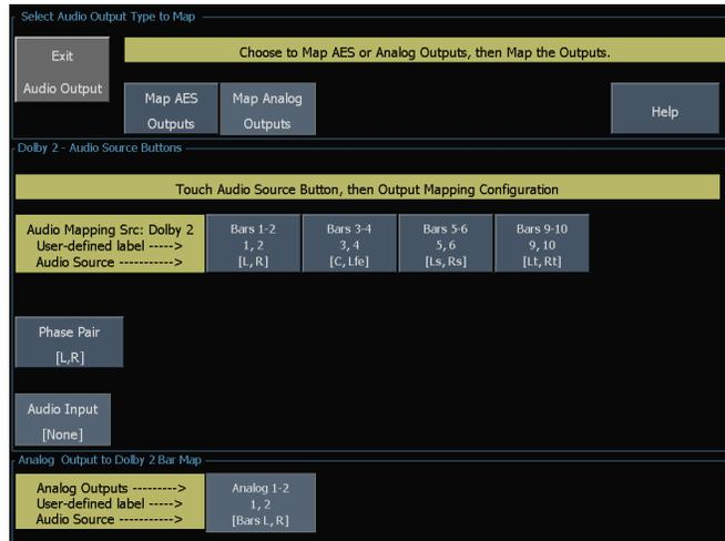
8. **Option DDE only:** Select the **Map AES Output** and assign specific bar pairs to the AES outputs in the map that appears. The AES bank must be configured as outputs. To route the undecoded Dolby Digital or Dolby E source to the AES outputs, select the **Undecoded source** button and then select the desired AES output
