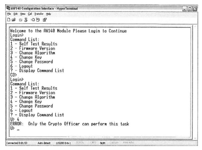
**Self Test Results** displays the results of the power up self test. At power up, the XPress<sup>™</sup> Crypto Module runs a known answer test for all encryption/decryption algorithms.
