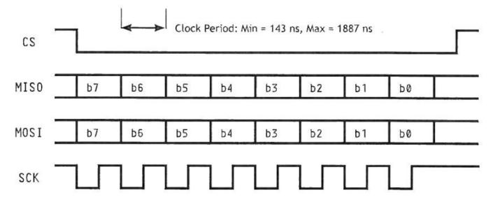
The SPI operates in slave mode, meaning SCK is supplied by an external source. This interface is used to transfer data to and from the module and to read status information.
