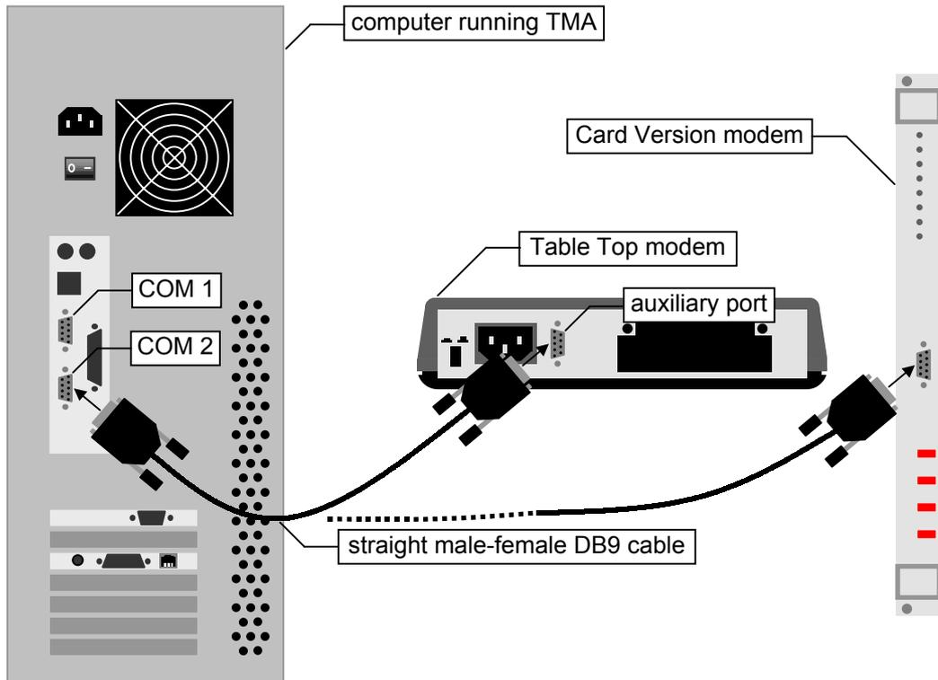
Once the connection is made then the computer running TMA is able to reach the modem.
