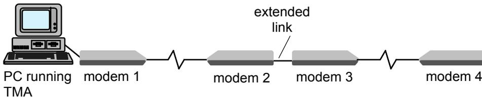
Your computer running TMA is connected on COM1 via a direct connection to the control port of modem 1. So, in the *Connect... – Device...* window you select Serial: com1, enter a *Password* if necessary and press on the *Next* button.
