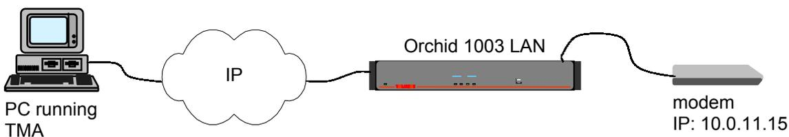
Your computer running TMA is connected over an IP network to an Orchid 1003 LAN. One of the ports of the Orchid is connected to the control port of a modem. This modem is configured in the object table of the Orchid. It is assigned IP address 10.0.11.15. So, in the *Connect... – Device...* window you select IP address: 10.0.11.15, enter a *Password* if necessary and press on the *Next* button.
