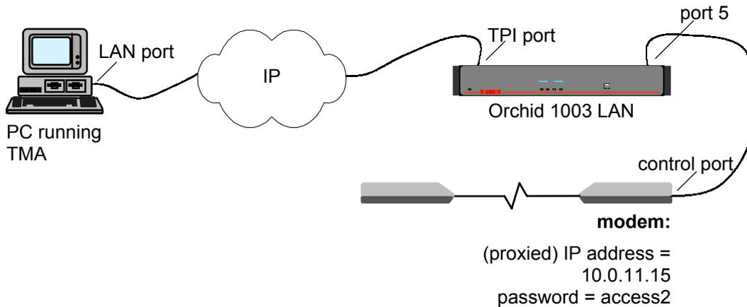
Suppose you want to open a TMA session on the modem. In this example, the Orchid 1003 LAN acts as an IP proxy device for the modem. I.e. the modem is configured in the object table of the Orchid 1003 LAN (IP address, exit port, etc.). For more information, refer to [Section 3.4 - Proxied IP connection to a non-IP device](#).
