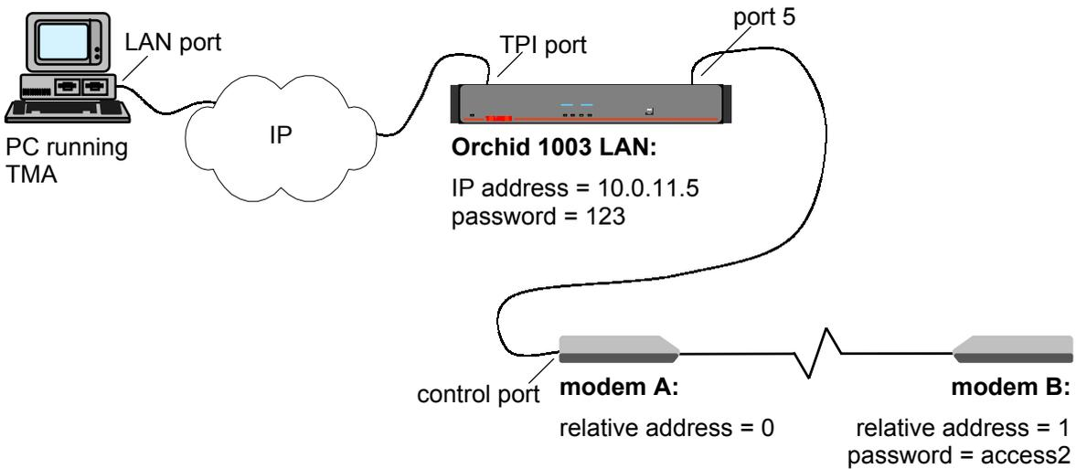
Suppose you want to open a TMA session on modem B. In this example, both modem A and B are configured in the object table of the Orchid 1003 LAN. However, they are not assigned an IP address. I.e. you can not connect to the modem over a proxied IP connection. You have to connect over IP to the Orchid first.
