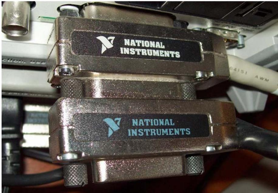
Figure 1. GPIB Chain Connection
