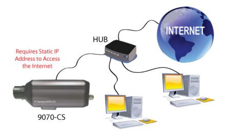
In this case, the 9070-IR is being connected to the internet through a hub, which is different from a router. The hub does not provide DHCP, and therefore would require that this setup have a static IP Address that is provided by the ISP.
