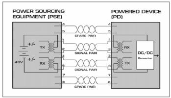
Power can be sourced from the PSE through the data lines via data transformer center taps
