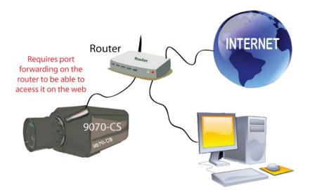
In this case, the 9070-IR will need to be port forwarded on the router so that it can accessed by the internet.
